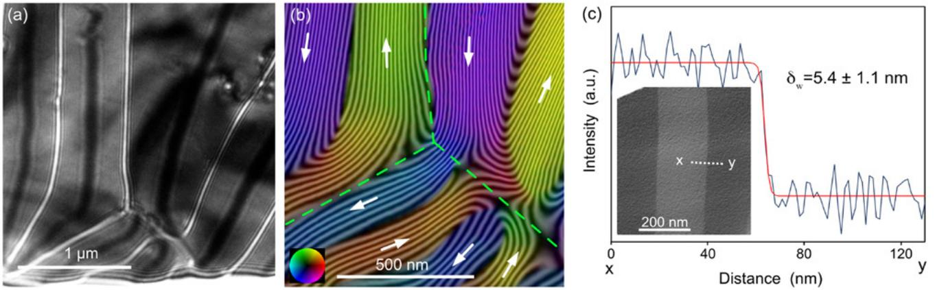
Fig 1: Magnetic imaging studies of the grain-boundary diffusion processed Nd-Fe-B magnet
