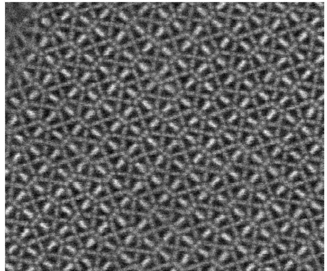
Fig. 2: Atomic resolution Z-contrast image of a  $Nd_2Fe_{14}B$  crystal grain viewed in the [001] zone axis
