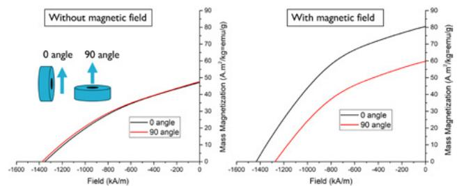
Fig 5: Magnetic properties of ring-shaped magnets with and without external magnetic field
