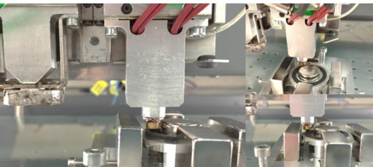
Fig 6: Printing of ring-shaped magnets
