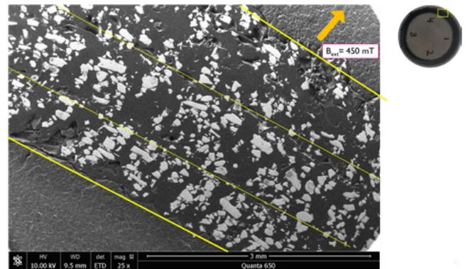
Fig 7: Particle Alignment due to the external magnetic field during printing process
