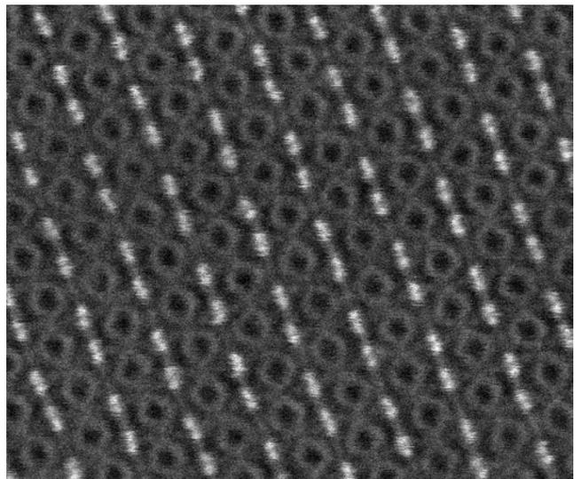
Fig. 3: Atomic resolution Z-contrast image of a  $Nd_2Fe_{14}B$  crystal grain viewed in the [100] zone axis
