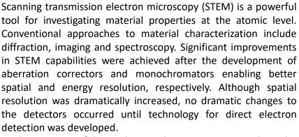
Implementation of direct electron detectors in STEM, where the whole diffraction pattern is recorded, facilitated the development of a new imaging technique - 4D STEM. A fundamental idea behind 4D STEM is a simultaneous acquisition of big data sets that are processed into distinct signals that uncover various physical material properties resulting in high-resolution images of charge densities, magnetization, strain maps, light elements etc.
