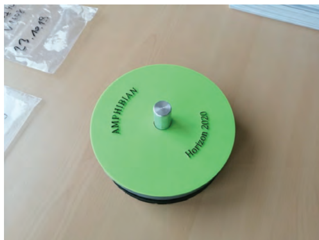
Figure 3: Flywheel prototype in which Nd-Fe-B magnets were replaced by ferrite magnets.
