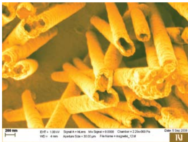
Figure 1: Co-Pt-based tubular structures synthesised with direct electroplating (left). Magnetic properties of the as-deposited Co-Pt-based nanotubes and the heat treated Co-Pt-based nanotubes (right).
