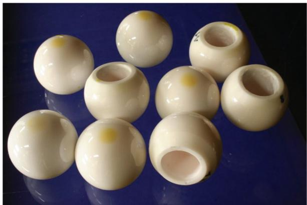
Figure 2: Test series of ceramic ball-heads for hip joints with a gradient composition were produced in the frame of the European project "Biograd". ([http://cordis.europa.eu/fetch?CALLER=OFFR\\_TM\\_EN&ACTION=D&DOC=2&CAT=OFFRE&QUERY=1197645527573&RCN=3420](http://cordis.europa.eu/fetch?CALLER=OFFR_TM_EN&ACTION=D&DOC=2&CAT=OFFRE&QUERY=1197645527573&RCN=3420))
